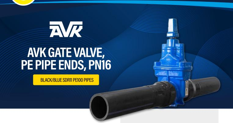
AVK gate valves are designed with built-in safety in every detail. The wedge is fully vulcanized with AVK's own drinking water approved EPDM rubber compound. It features an outstanding durability due to the ability of the rubber to regain its original shape, the double bonding vulcanization process and the sturdy wedge design. The triple safety stem sealing system, the high strength stem and the thorough corrosion protection safeguard the unmatched reliability.
